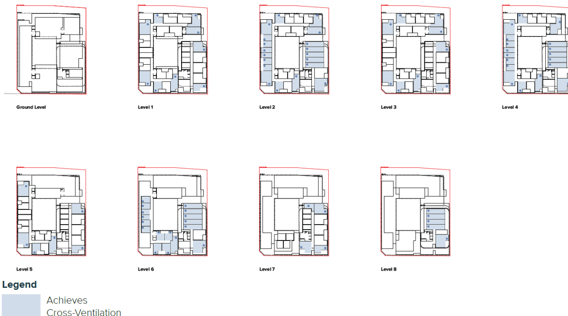
Figure 44 | Typical floor plan and achievement of cross ventilated apartments in first 9 storeys for buildings on Lot S
